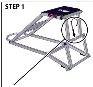
Raise the lift to the position shown above and insert the safety pin provided. This will position the lift in approximately the correct position for the foot pedal assembly.
