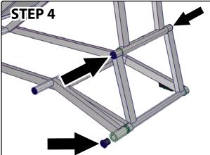
Use a hammer or mallet to install the 3 plastic end cap into the open holes in the lift as shown above. Remove the safety pin and read the instructions on how to properly use the lift. Wrap the safety pin around the upper side bar above the front graphic plate so it doesn't get lost while not in use.
