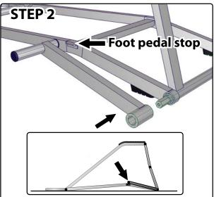
When the lift is locked in place with the safety pin, place the foot pedal on the hex shaft at the angle shown. The end of the foot pedal should rest on the foot pedal stop.
